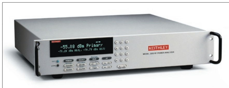
Figure 1: The RF power analyzer is meant for production test of mobile phones. It works only at cell phone frequencies, and it measures only those parameters that are required for cell phone testing: carrier frequency, primary channel power, upper and lower adjacent channel power, and upper and lower alternate channel power.
